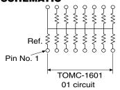
The 01 circuit provides 15 nominally equal resistors, each connected between a common lead (16) and a discrete PC board pin.
